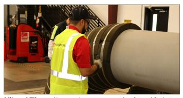
**Mitered Elbows**: Narrow pieces are more fragile and likely to damage in transport. The mitered system also creates more joints and reduces thermal protection.
