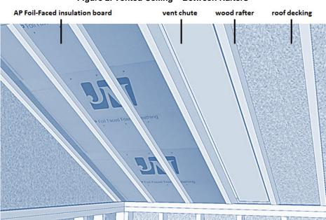
Figure 2. Vented Ceiling – Between Rafters
