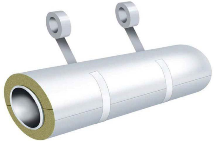
FIGURE 6: TAPING PATTERN FOR CHILLED WATER APPLICATIONS
